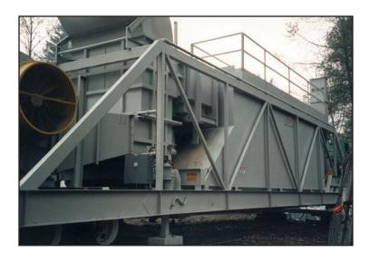
trailer, and Terra Therm markets it. Employing so-called In Situ Thermal Desorption (ISTD) technology, the system remediates a broad range of organic compounds such as PCBs, pesticides, petroleum wastes, and chlorinated solvents, all without excavating the soil.
