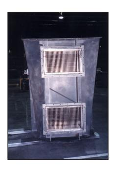
the Thermo-Z, they capture heat from the flue gases coming out of the liquid heater's exhaust at 680°F and use it to preheat combustion air going into the heater at 365°F. The heat exchanger increases the efficiency of the heater by 10%, saving the customer an equivalent amount in fuel.
