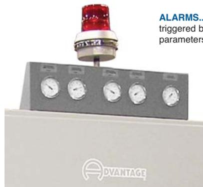
**ALARMS...** Audible and visual alarms are triggered by process temperature and pressure parameters, factory or operator set.
