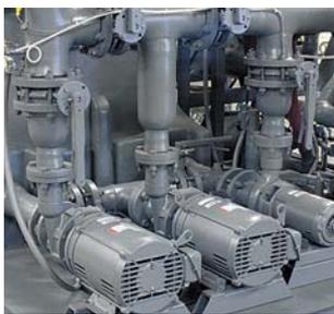
Titan® central chillers use a 2-pump system... one pump to deliver coolant flow to process and a second pump to deliver coolant flow through the chiller evaporators. The process and evaporator pumps operate independently of each other, allowing for greater control of coolant temperature, flow and pressure. Each pump is toggled on and off by individual operators.
