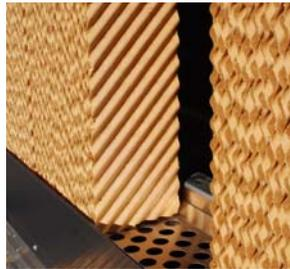
When evaporative pre-cooling is required, a highly absorbent media is wet using city water. The honeycomb design provides a large wetted surface that is exposed to the entering air to provide maximum adiabatic effect to lower the incoming air temperature. 6" thick media is used to provide the required performance. Excess water
