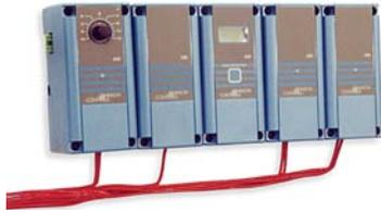
**MULTISTAGE CONTROLLER...** stages tower fans and tower pumps to match system capacity to the cooling load. This panel mounted control package maintains a consistent water temperature regardless of load and ambient conditions. The electronic thermostat features a digital set point and a digital readout of actual water temperature. A single set point value is entered and offsets stage fans, pumps and alarms are staged appropriately... no need to set individual thermostats.
