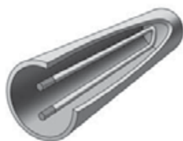
FIG. N - Pipe wells
