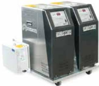
Processors often want to run different temperatures on each mold half to produce the best part quality. A dual zone dolly that holds two standard single zone units adds convenience by providing a common castered dolly with optional single cooling water supply and drain connection and optional electrical junction box where both units can be connected with a single power supply.
