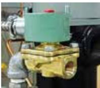
A standard feature of all units with the VE or 300°F controller is the solenoid controlled cooling valve. Pulsed by the microprocessor controller, the solenoid cooling valve provides good temperature control and is best applied on applications with small cooling loads and when a large temperature difference exists between the set point and cooling water temperatures.
